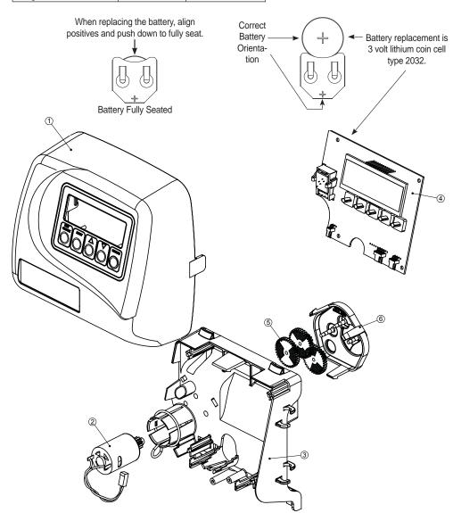
WS1 Drive Cap Assembly, Downflow Piston, Upflow Piston, Regenerant Piston and Spacer Stack Assembly
