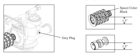
WS1.25 with 32mm Distributor Tube Opening Identification
